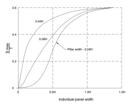
Fig. 4.1 Graph for the Prediction of Maximum Subsidence over a Series of Panels for Critical Extraction Conditions (after Holla, 1988)
