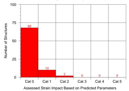
Fig. 5.3 Distribution of the Assessed Strain Impacts for the Rural Building Structures within the Study Area Based on the Predicted Systematic Subsidence Parameters
