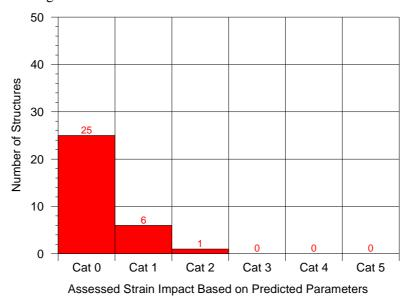
Fig. 5.13 Distribution of the Assessed Strain Impacts for the Houses within the Study Area Based on the Predicted Systematic Subsidence Parameters
