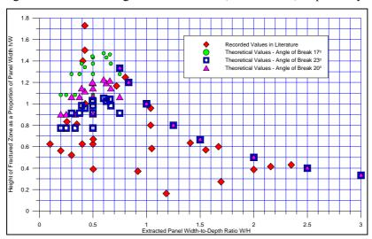
Fig. 5.17 Graph showing Height of Fractured Zone as a Proportion of Panel Width for different Width-to-Depth Ratios
