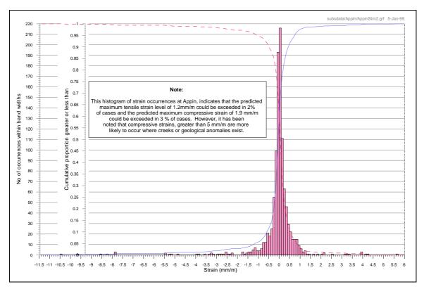
Fig. 4.2 Distribution of Measured Strains at Appin Colliery
