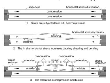
Fig. D.25 Strata Buckling Mechanism due to In-situ Horizontal Stress
