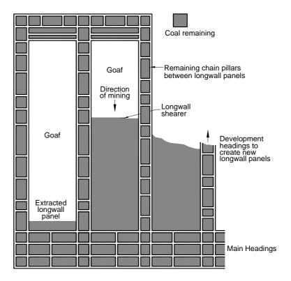
Fig. C.4 Typical Plan View of a Series of Longwall Panels
