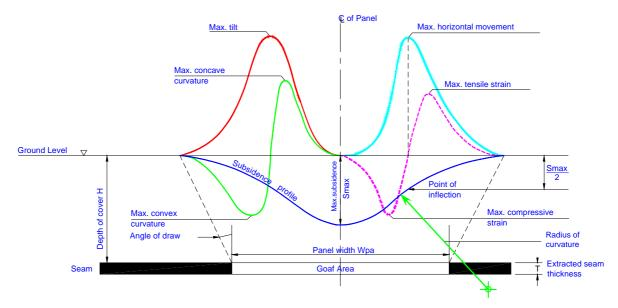
Fig. 3.2 Typical Profiles of Systematic Subsidence Parameters for a Single Longwall Panel
