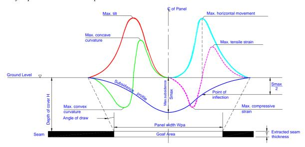
Fig. C.6 Subsidence Parameter Profiles above a Single Longwall Panel
