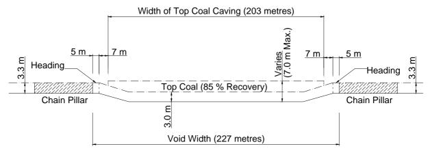
Fig. 3.1 Cross-Section through a Typical Proposed Austar Longwall A6 to A17
