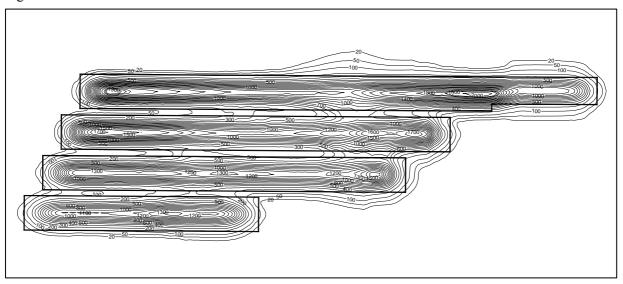
Fig. D.6 Typical Predicted Subsidence Contours over a Series of Longwalls
