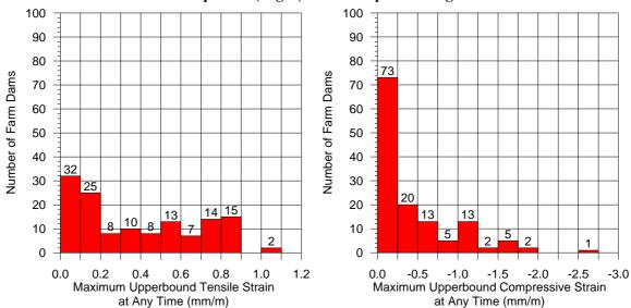
Fig. 5.10 Maximum Upperbound Systematic Tensile Strain (Left) and Compressive Strain (Right) at the Farm Dams Resulting from the Extraction of the Proposed Longwalls
