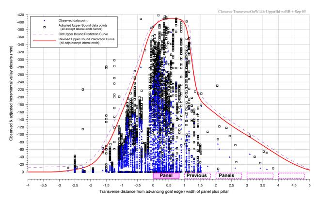
Fig. D.12 Valley Closure versus Distance from the Advancing Goaf Edge of the Longwall relative to the Width of the Panel plus the Width of the Pillar
