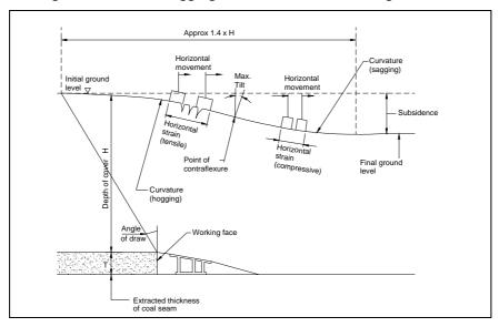
Fig. C.7 Development of a Subsidence Trough (to an exaggerated vertical scale)
