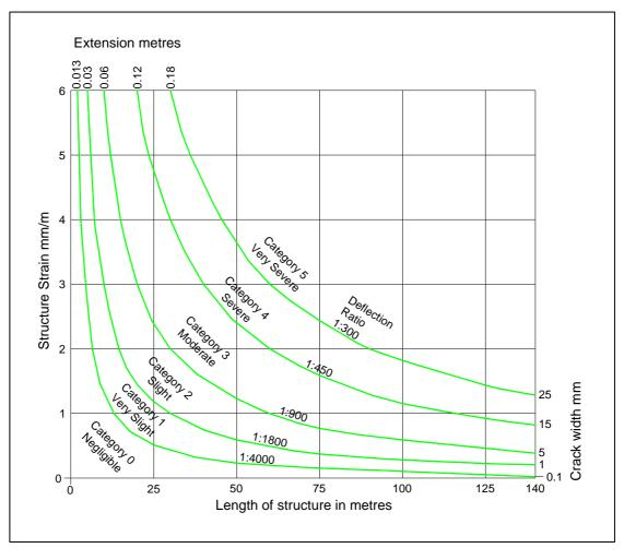
Fig. E.2 Impact Classification with Deflection Ratios for Two Storey Brick Structures
