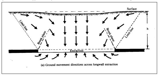
Fig. D.9 Normal Mining Induced Movements above an Extracted Area (after Whittaker, Reddish and Fitzpatrick, 1985)
