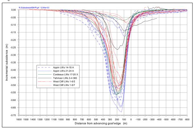
Fig. D.2 Typical Incremental Subsidence Profiles – NSW Southern Coalfield
