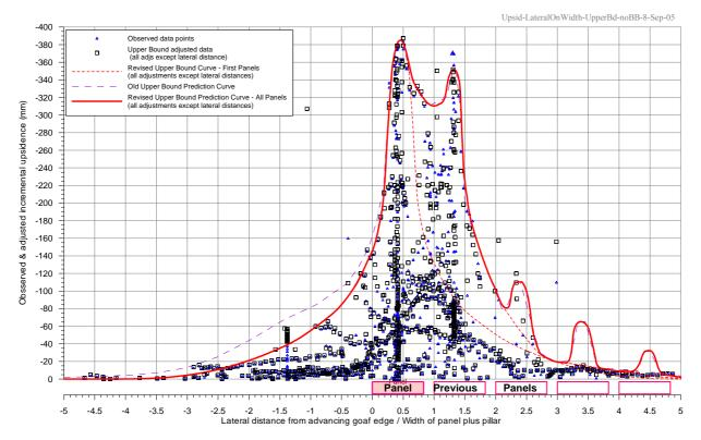
Fig. D.17 Upsidence versus Distance from the Advancing Goaf Edge of the Longwall relative to the Width of the Panel plus the Width of the Pillar
