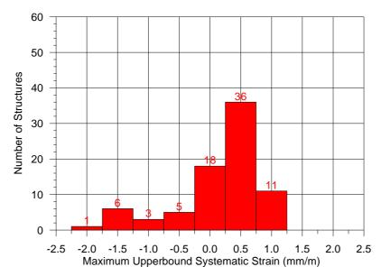
Fig. 5.2 Distribution of the Maximum Upperbound Systematic Strains at the Rural Building Structures within the Study Area Resulting from the Extraction of the Proposed Longwalls
