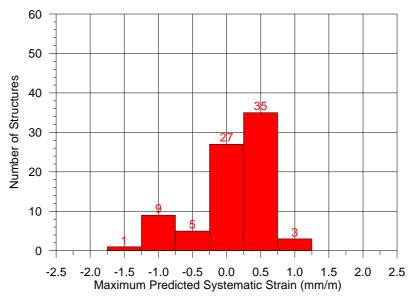
Fig. 5.1 Distribution of the Maximum Predicted Systematic Strains at the Rural Building Structures within the Study Area Resulting from the Extraction of the Proposed Longwalls
