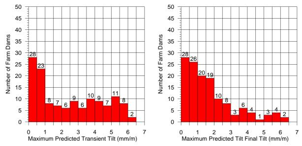
Fig. 5.6 Maximum Predicted Travelling and Cumulative Tilt (Left) and Maximum Predicted Total Tilt (Right) at the Farm Dams Resulting from the Extraction of the Proposed Longwalls
