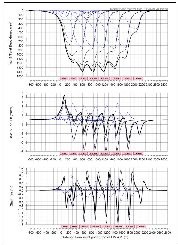
Fig. D.5 Typical Predicted Incremental and Total Subsidence, Tilt and Strain Profiles
