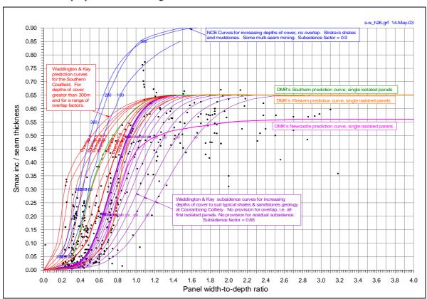
Fig. 3.5 Maximum Observed Subsidence in the New South Wales Coalfields
