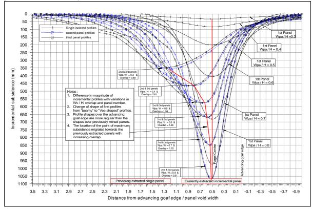
Fig. D.3 Incremental Subsidence Profiles obtained using the Incremental Profile Method
