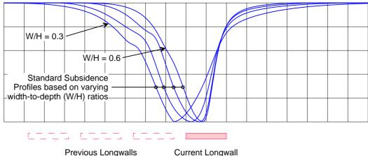
Fig. 3.4 Standard Normalised Profiles based on Varying Width-to-Depth Ratios
