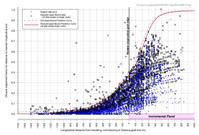
Fig. D.13 Valley Closure Adjustment Factor versus Longitudinal Distance
