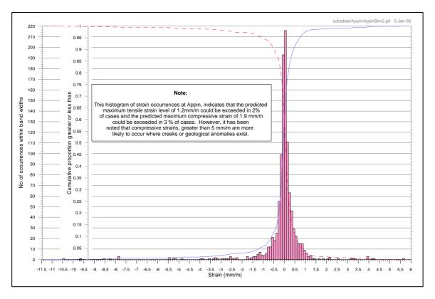
Fig. D.7 Graph showing Histogram of Strain Occurrences at Appin Colliery
