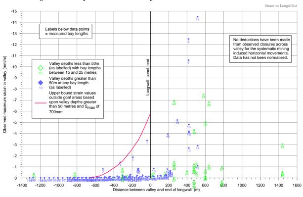
Fig. D.24 Graph of Maximum Compressive Strain versus Longitudinal Distance
