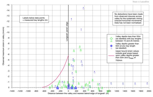
Fig. D.23 Graph of Maximum Compressive Strain versus Lateral Distance
