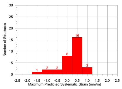
Fig. 5.11 Distribution of the Maximum Predicted Systematic Strains at the Houses within the Study Area Resulting from the Extraction of the Proposed Longwalls
