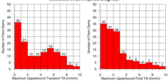
Fig. 5.9 Maximum Upperbound Systematic Tilt at the Farm Dams at Any Time (Left) and at the Completion (Right) of the Proposed Longwalls
