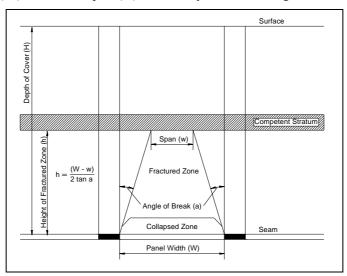
Fig. 5.16 Theoretical Model illustrating the Development and Limit of the Fractured Zone
