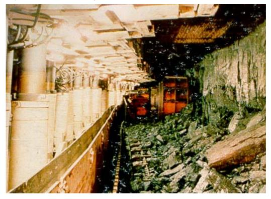
Fig. C.3 Typical Longwall Face Equipment
