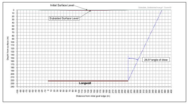
Fig. C.5 Typical Subsidence Profile Drawn to a True Scale
