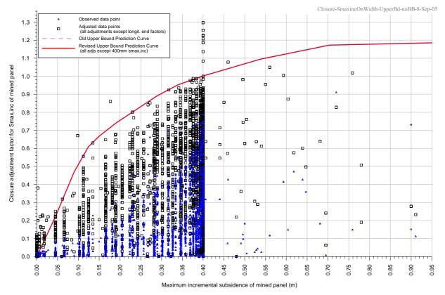
Fig. D.15 Valley Closure Adjustment Factor versus Maximum Incremental Subsidence
