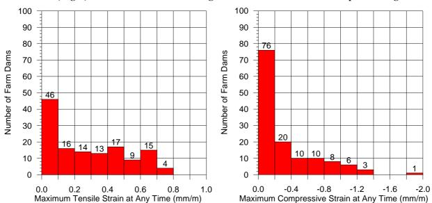
Fig. 5.7 Maximum Predicted Systematic Tensile Strain (Left) and Compressive Strain (Right) at the Farm Dams Resulting from the Extraction of the Proposed Longwalls
