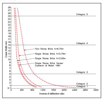
Fig. E.4 Variation of Crack Width with Deflection Ratio for Brick Structures
