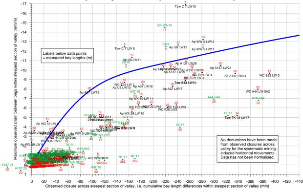
Fig. D.22 Graph of Maximum Compressive Strain versus Valley Closure
