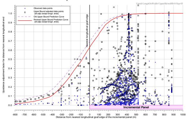
Fig. D.18 Upsidence Adjustment Factor versus Longitudinal Distance
