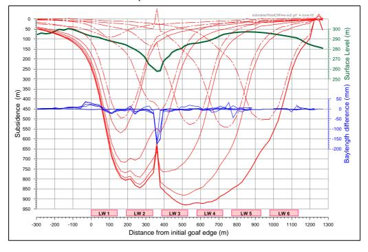
Fig. D.11 Measured Subsidence Profiles over Longwalls 1 to 6 at West Cliff Colliery
