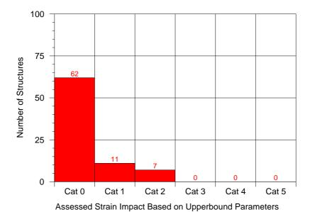
Fig. 5.4 Distribution of the Assessed Strain Impacts for the Rural Building Structures within the Study Area Based on the Upperbound Systematic Subsidence Parameters
