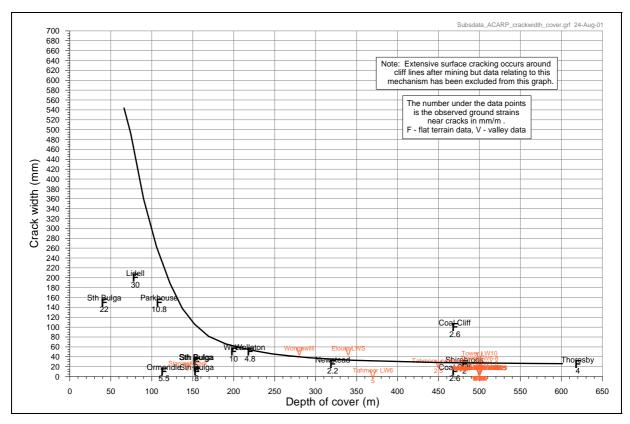
Fig. D.8 Relationship between Crack Width and Depth of Cover
