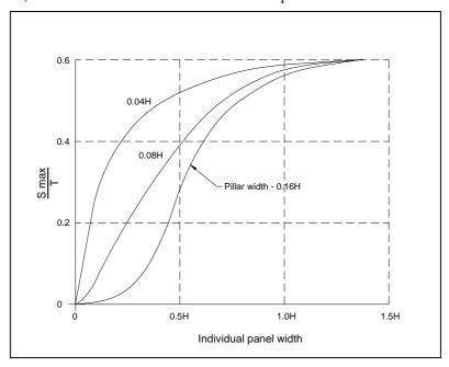
Fig. D.1 Graph for the Prediction of Maximum Subsidence over a Series of Panels for Critical Extraction Conditions (after Holla, 1988)
