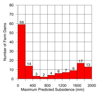
Fig. 5.5 Maximum Predicted Total Systematic Subsidence at the Farm Dams Resulting from the Extraction of the Proposed Longwalls
