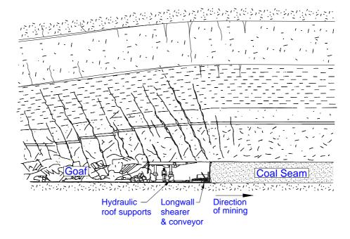
Fig. C.2 Cross Section of a Typical Longwall Face
