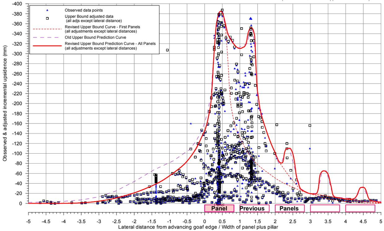
**Fig. D.17 Upsidence versus Distance from the Advancing Goaf Edge of the Longwall relative to the Width of the Panel plus the Width of the Pillar**
