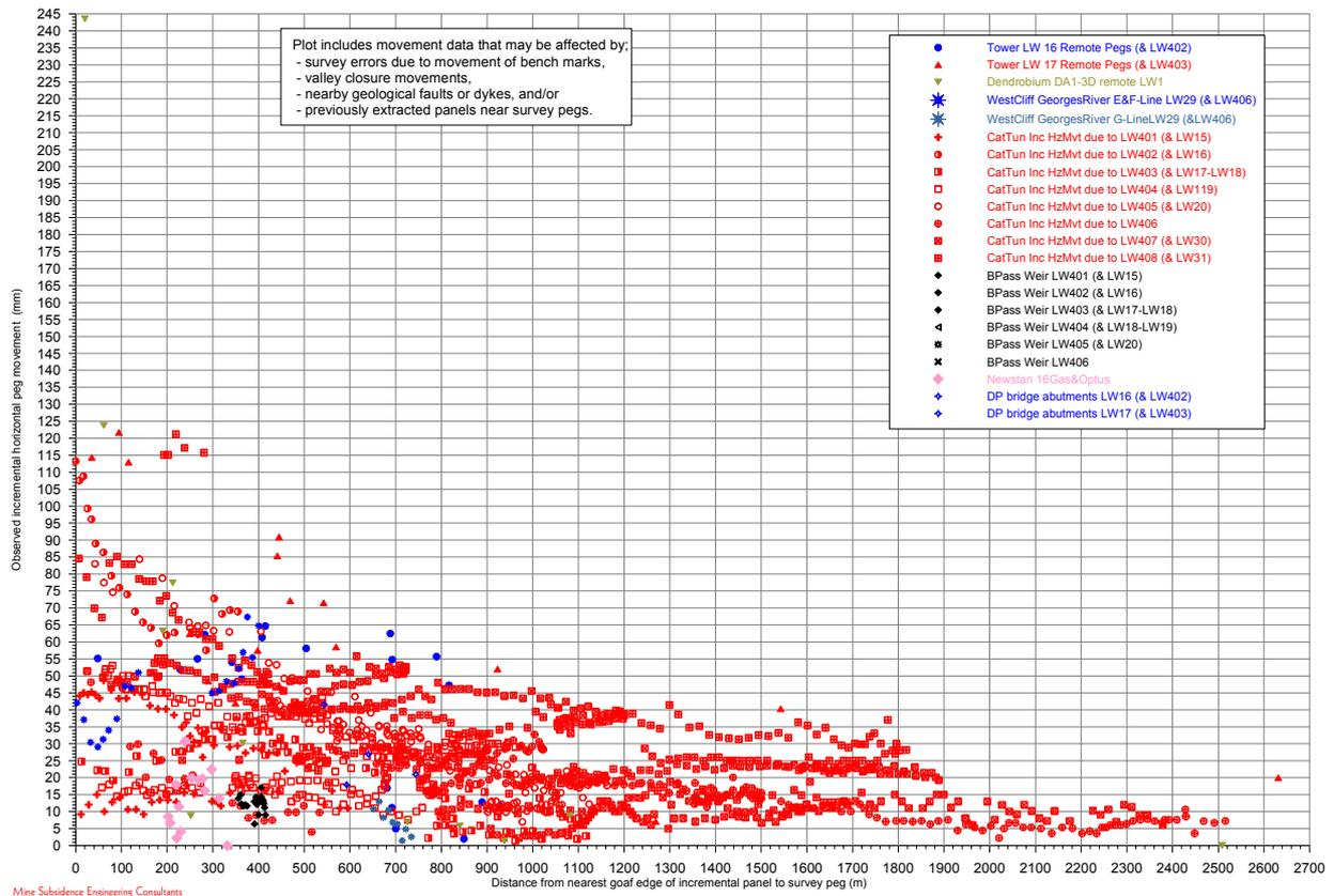
**Fig. D.27 Observed Incremental Regional Horizontal Movements with Solid Coal between the Monitoring Points and Mined Longwall**
