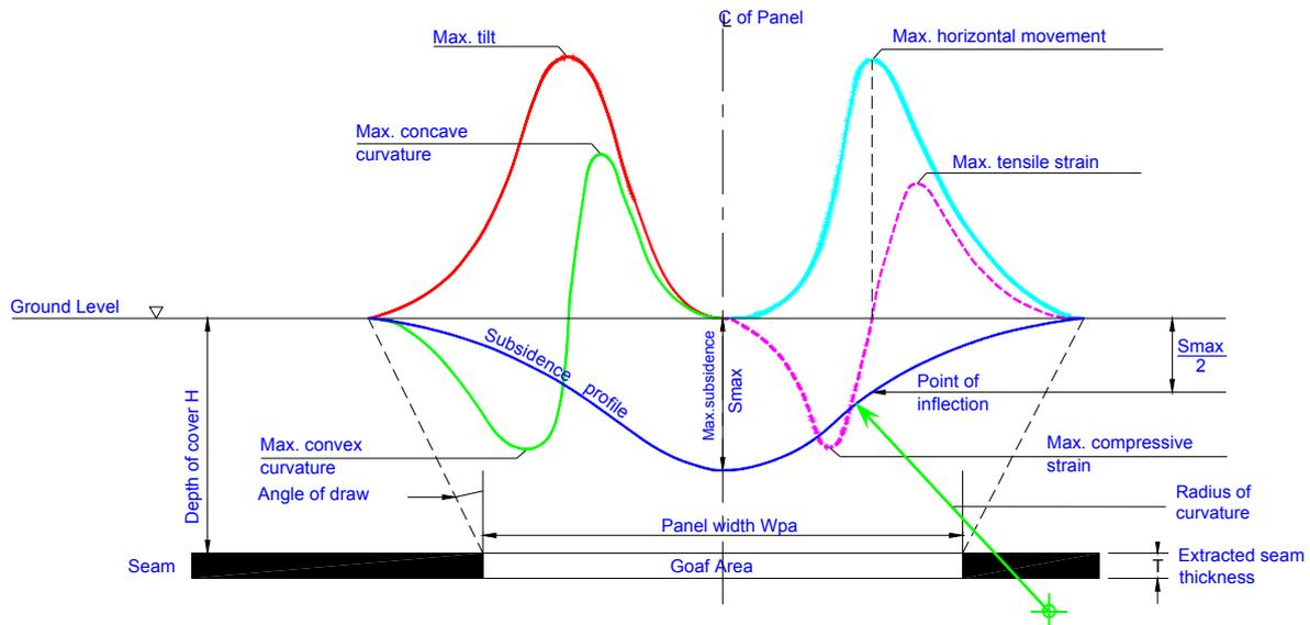
**Fig. 3.2 Typical Profiles of Systematic Subsidence Parameters for a Single Longwall Panel**
