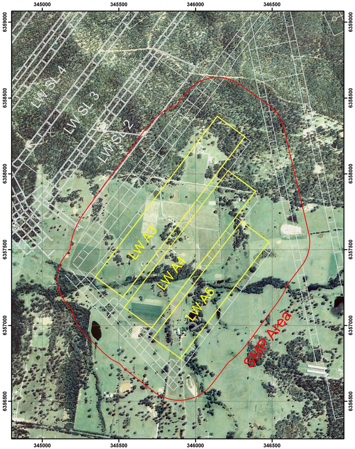
**Fig. 1.1 Aerial Photograph Showing the Proposed Longwalls and the SMP Area**
