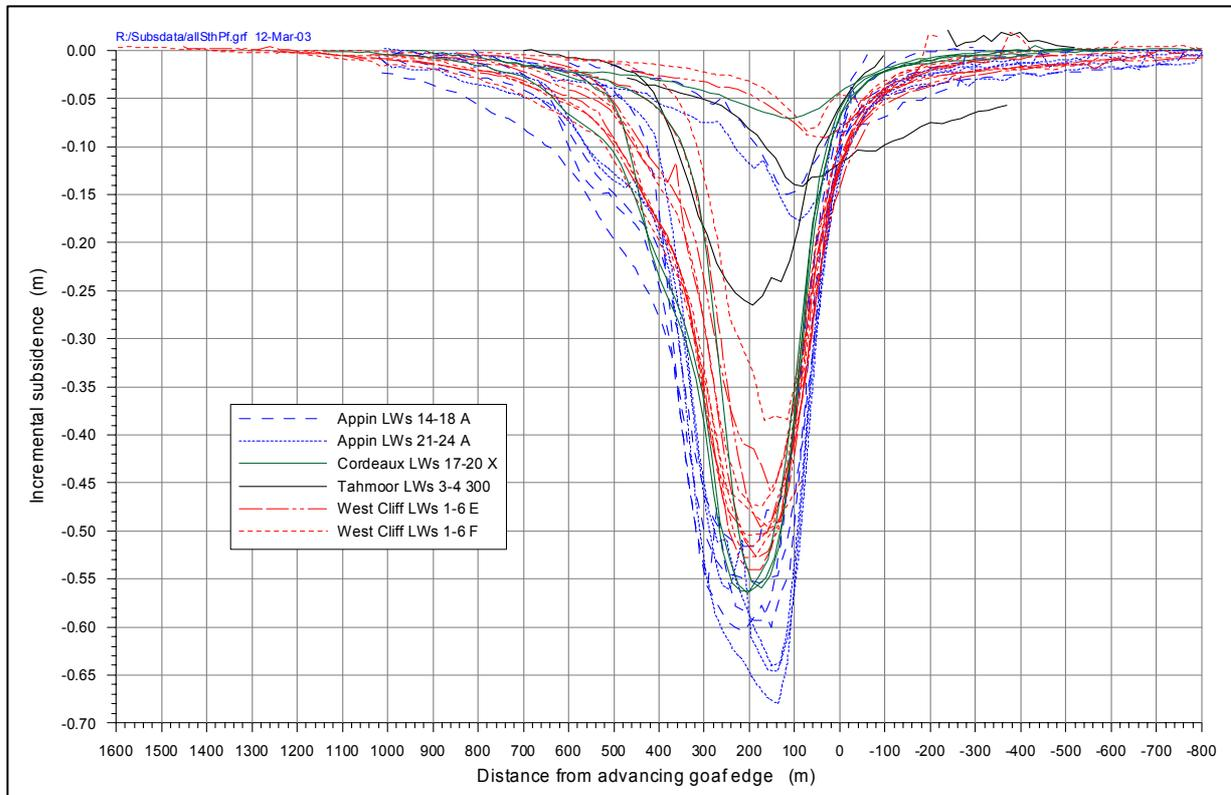
**Fig. D.2 Typical Incremental Subsidence Profiles – NSW Southern Coalfield**
