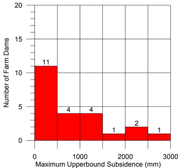
**Fig. 5.4 Maximum Upperbound Systematic Subsidence at the Farm Dams after the Extraction of the Proposed Longwalls A3 to A5**
