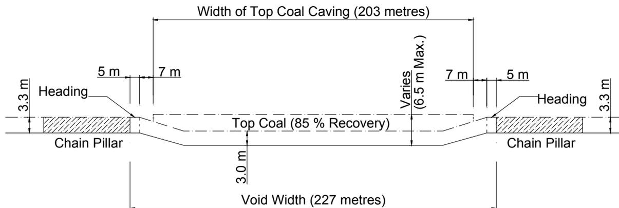
**Fig. 3.1 Cross-Section through a Typical Proposed Austar Longwall A3 to A5**
