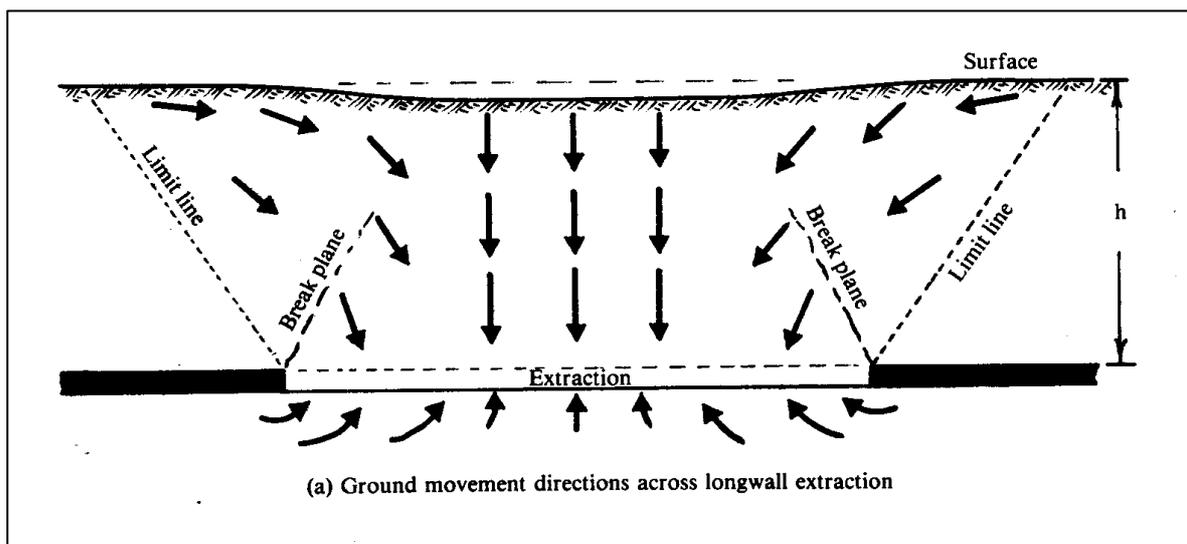
**Fig. D.9 Normal Mining Induced Movements above an Extracted Area (after Whittaker, Reddish and Fitzpatrick, 1985)**
