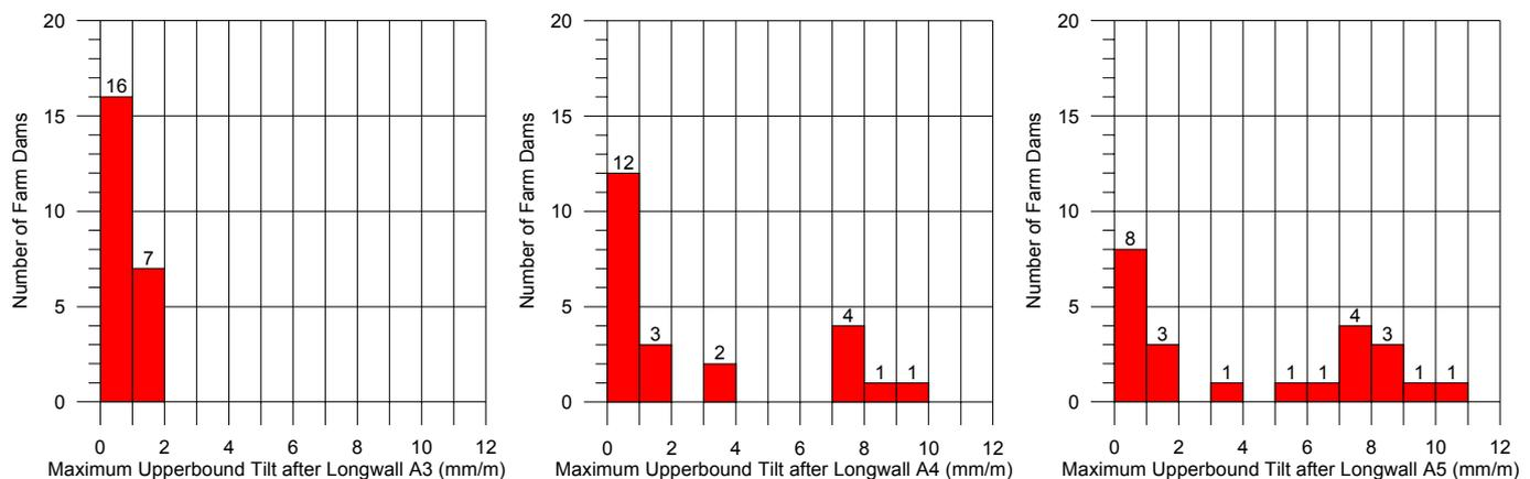
**Fig. 5.5 Maximum Upperbound Systematic Tilt at the Farm Dams after the Extraction of Proposed Longwall A3 (Left), Proposed Longwall A4 (Middle), and Proposed Longwall A5 (Right)**
