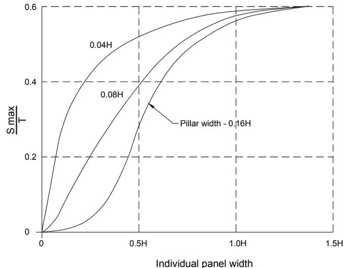
**Fig. 5.9 Graph for the Prediction of Maximum Subsidence over a Series of Panels for Critical Extraction Conditions (after Holla, 1988)**
