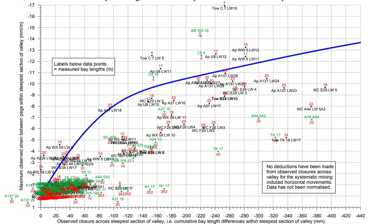
**Fig. D.22 Graph of Maximum Compressive Strain versus Valley Closure**
