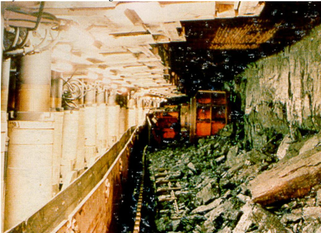
**Fig. C.3 Typical Longwall Face Equipment**
