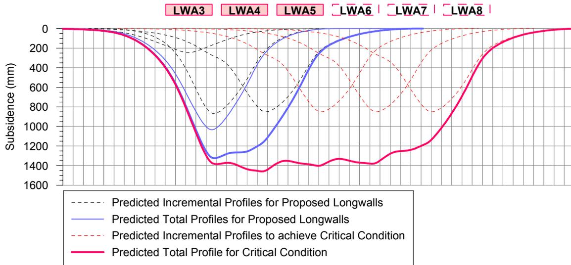
**Fig. 5.10 Maximum Predicted Total Subsidence for Critical Conditions Obtained Using the Incremental Profile Method**
