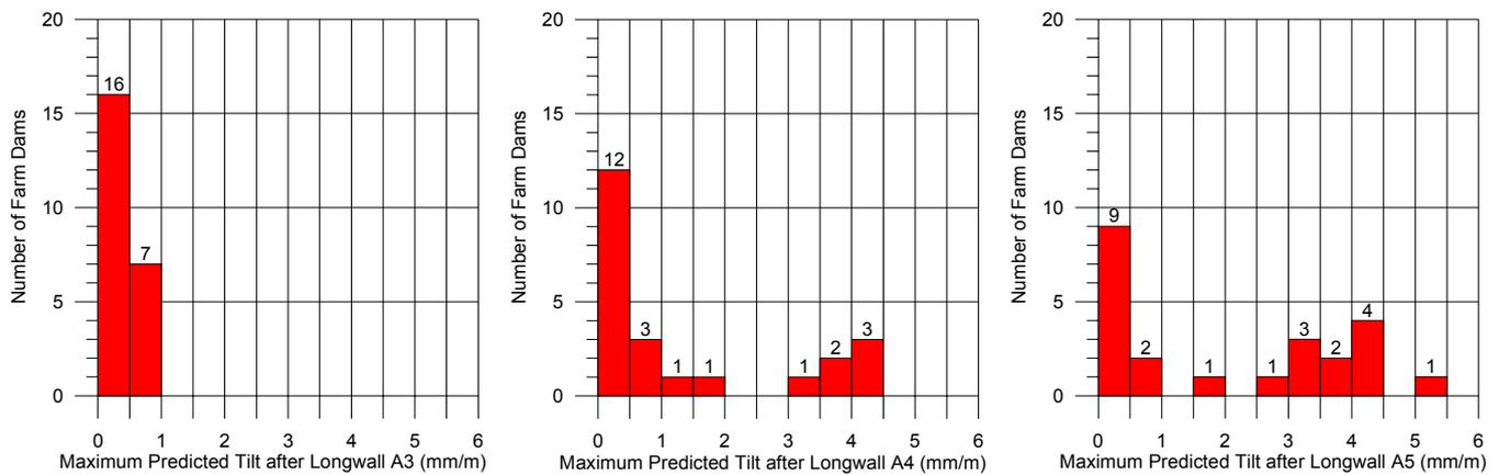
**Fig. 5.2 Maximum Predicted Systematic Tilt at the Farm Dams after the Extraction of Proposed Longwall A3 (Left), Proposed Longwall A4 (Middle), and Proposed Longwall A5 (Right)**
