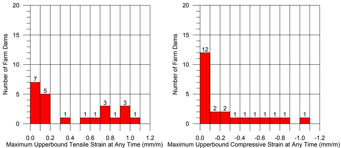
**Fig. 5.6 Maximum Upperbound Systematic Tensile Strain (Left) and Compressive Strain (Right) at the Farm Dams Resulting from the Extraction of Proposed Longwalls A3 to A5**
