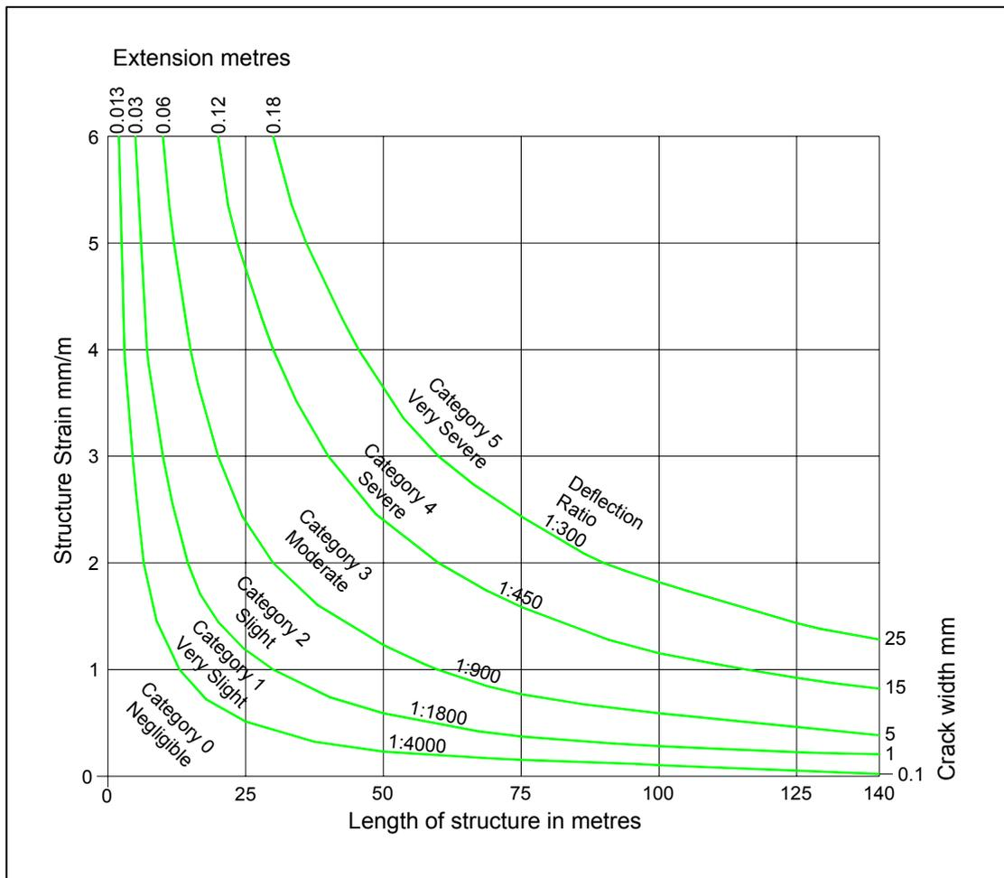
**Fig. E.2 Impact Classification with Deflection Ratios for Two Storey Brick Structures**
