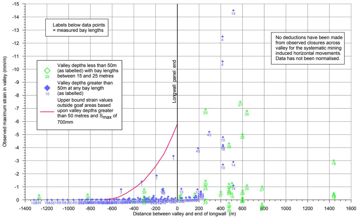
**Fig. D.24 Graph of Maximum Compressive Strain versus Longitudinal Distance**
