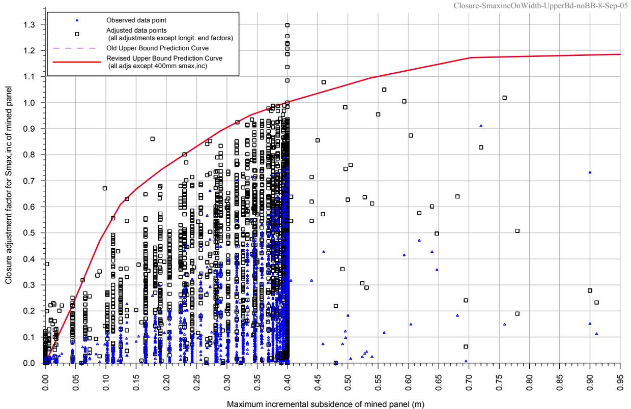
**Fig. D.15 Valley Closure Adjustment Factor versus Maximum Incremental Subsidence**
