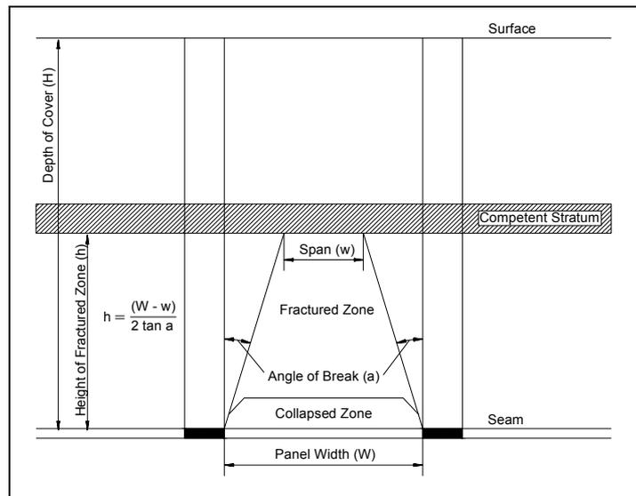
**Fig. 5.7 Theoretical Model illustrating the Development and Limit of the Fractured Zone**
