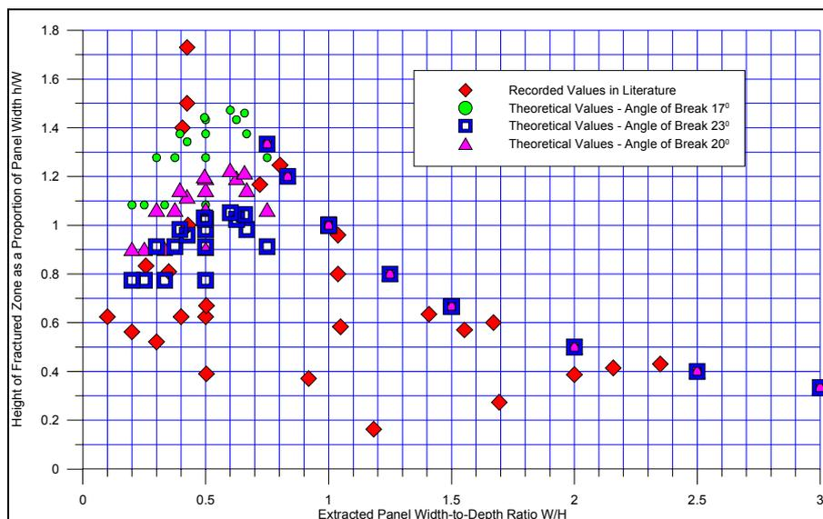
**Fig. 5.8 Graph showing Height of Fractured Zone as a Proportion of Panel Width for different Width-to-Depth Ratios**
