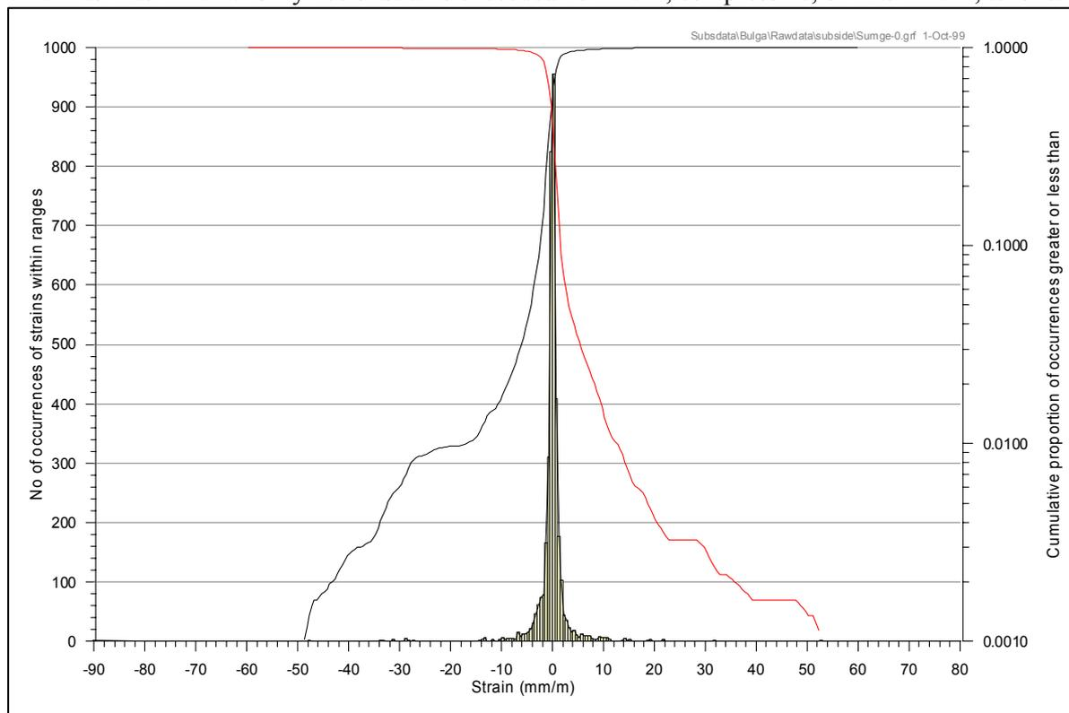
**Fig. D.7** Graph showing Histogram of Strain Occurrences at South Bulga Colliery
