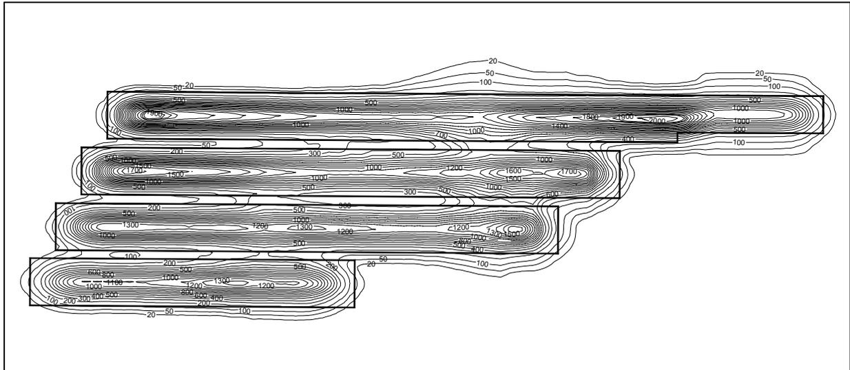
**Fig. D.6 Typical Predicted Subsidence Contours over a Series of Longwalls**
