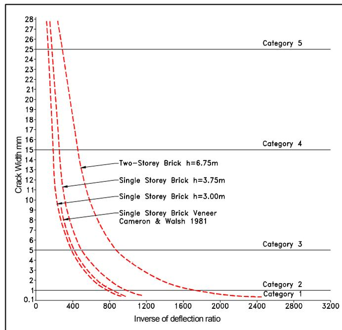
Fig. E.4 Variation of Crack Width with Deflection Ratio for Brick Structures
