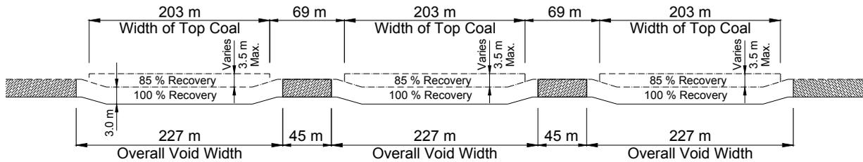
**Fig. 3.6 Cross-section through the Proposed Longwalls A3 to A5**
