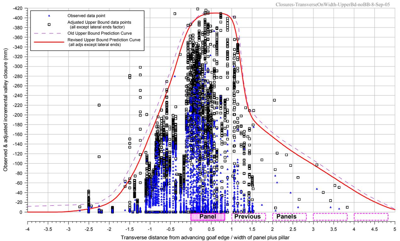
**Fig. D.12 Valley Closure versus Distance from the Advancing Goaf Edge of the Longwall relative to the Width of the Panel plus the Width of the Pillar**
