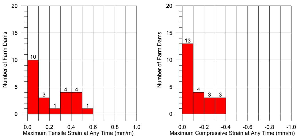
**Fig. 5.3 Maximum Predicted Systematic Tensile Strain (Left) and Compressive Strain (Right) at the Farm Dams Resulting from the Extraction of Proposed Longwalls A3 to A5**
