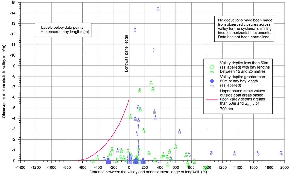
**Fig. D.23 Graph of Maximum Compressive Strain versus Lateral Distance**
