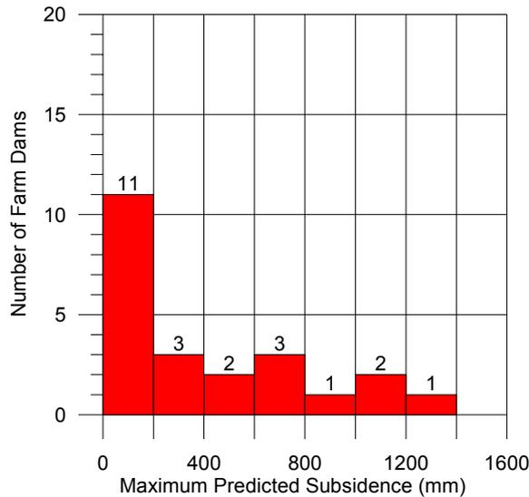
**Fig. 5.1 Maximum Predicted Systematic Subsidence at the Farm Dams after the Extraction of the Proposed Longwalls A3 to A5**
