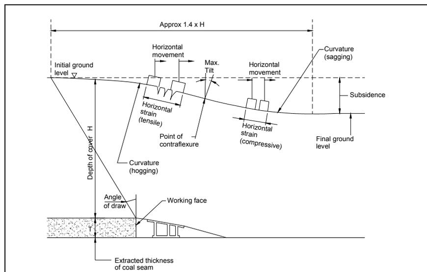
**Fig. C.7 Development of a Subsidence Trough (to an exaggerated vertical scale)**
