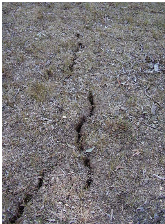
Fig. 4.5 Example of Surface Tensile Cracking in the Natural Ground Surface (Observed in the Southern Coalfield at a Similar Depth of Cover as the Study Area)
